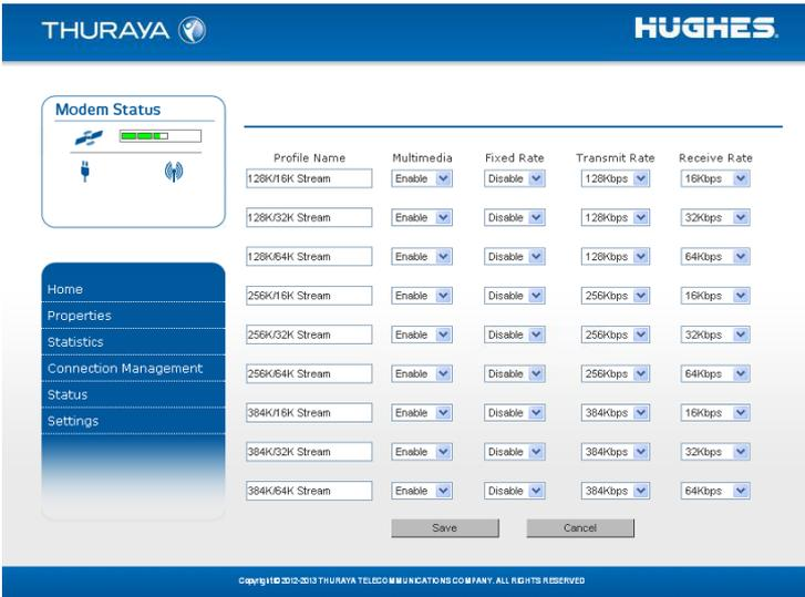
Accessible from the Main Menu, the **Connection Management Screen** allows you to select from nine Quality of Service (QoS) quick connect buttons. Each button can be customized using the **Details** link on the Connection Management Screen. The customization parameters for each button are as follows:
