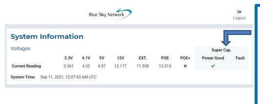
Data points about the supercapacitor (SC) can be found here.
