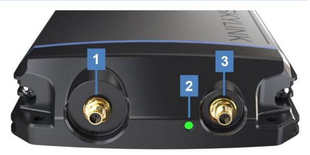
The top panel contains a power LED indicator and 2 connectors for an Iridium and cellular antenna. The descriptions below reference the photo above in accordance with the numerical value.
