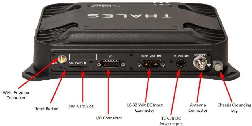
Gambar1-5Detail Panel Belakang Unit Terminal
