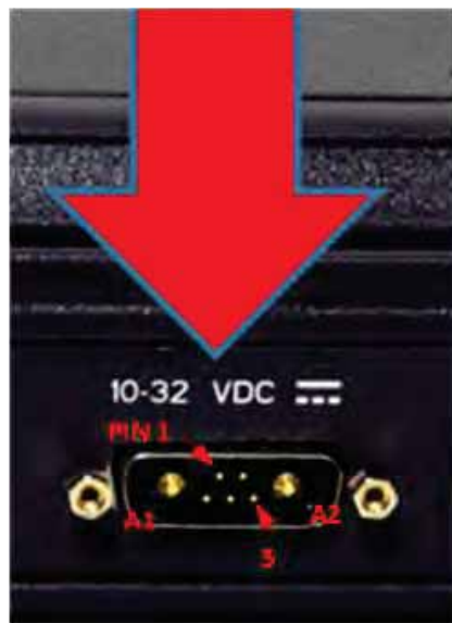
Figure 7-4 10-32 VDC and Mating Connector Detail
