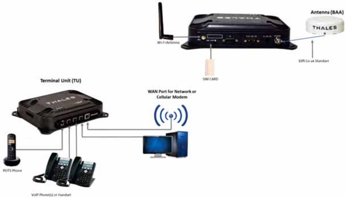
Figure 2-3 MissionLINK™ System with Connected Hardware
