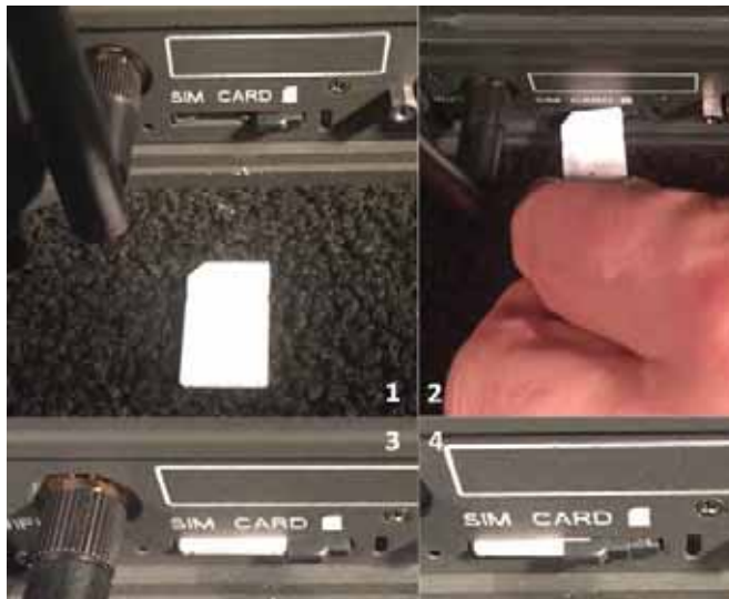
Figure 3-4 Installing SIM Card and Engaging the Lock
