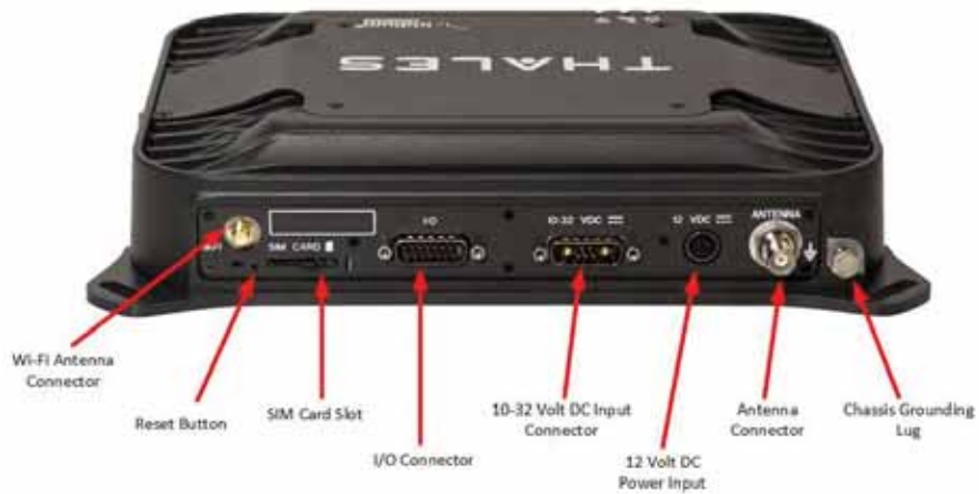
Figure 2-7 Terminal Unit (TU) Back Panel Detail
