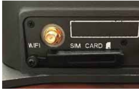
Figure 3-5 Secure the SIM Card Cover
