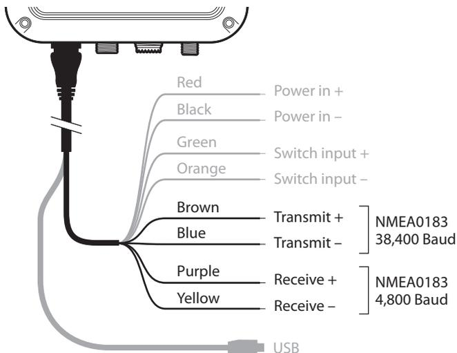
Figure 11 Connecting to the NMEA0183 data port
