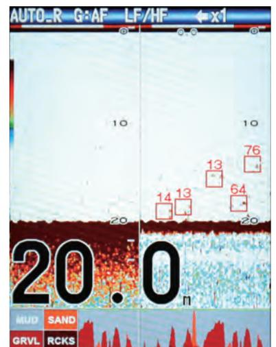
Circles or squares with fish sizes are displayed on fish echoes. When in dual frequencies mode, you can set the mark displayed on both or either frequency screen.
