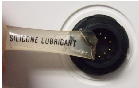
Figure 55 Silicone Lubricant and Connector
