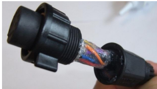
Figure 43 Silicone in the Grommet
